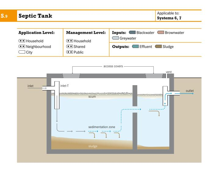
A septic tank is a watertight chamber made of concrete, fibreglass, PVC or plastic, through which blackwater and greywater flows for primary treatment. Settling and anaerobic processes reduce solids and organics, but the treatment is only moderate.
